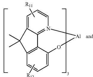
For example, for Al, x is 3 in this preferred embodiment, and the structure may be referred to as a "tris" structure. The tris structure is preferred because it is believed to be particularly stable.
