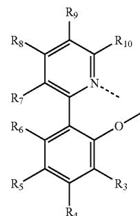
wherein the ligand is attached to a metal M, such that the resulting material has (i) an oxygen-metal bond and (ii) the nitrogen is coordinated to the metal;
